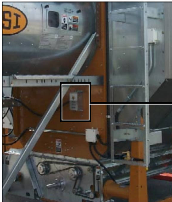
Air Switch location.
