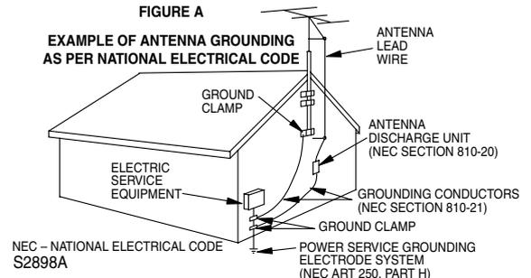
14. **Lightning-** For added protection for this video product during a lightning storm, or when it is left unattended and unused for long periods of time, unplug it from the wall outlet and disconnect the antenna or cable system. This will prevent damage to the video product due to lightning and power-line surges.
