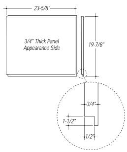
**1/4" Custom Panels** The GPF425 Trim Kit provides for the installation of 1/4" thick custom door and access panels.
