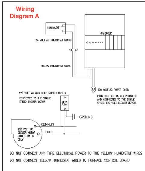
**11a. Wiring Diagram A: Single-Speed Blower.**
