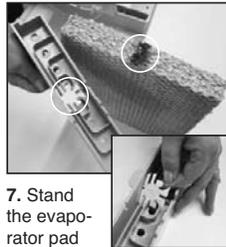
7. Stand the evaporator pad upright with the black index mark on top. Make sure the wick is seated securely in the drip tray.
