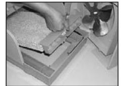
5. Pull out the drip tray and evaporator pad assembly by grasping the top lip and tipping out.
