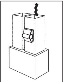
Mount the Model HUM-FP Fan-Powered Flow-Thru Humidifier on the **WARM AIR PLENUM ONLY**.
