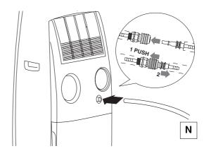
The water in the internal circuit will drain into the condensation tank (8) or through the continuous drain
