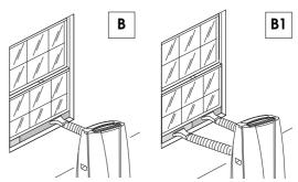
If the windows are large, use the window bar without holes (23) (if provided) to cover your window aperture, extending it to the required length, then blocking it with the locking pins supplied (see figure below). Make sure you do not cover the hole or holes for the window outlet.
