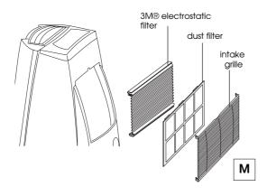
Use a vacuum cleaner to remove the dust collected on the filter.
