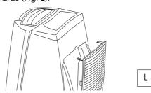
2. Remove the dust filter by detaching it from the grille (Fig. **M**). Remove 3M® electrostatic filter if it is mounted.
