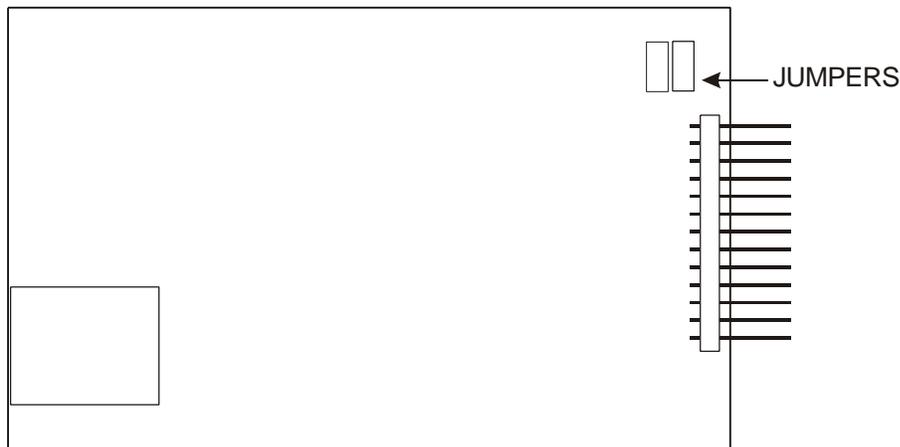
**Figure C-4 ISDN Module processor setting jumpers**
