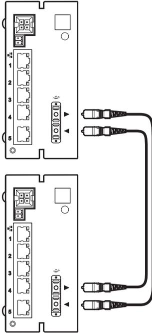
**Figure 7.** Fiber Port Connections in Point-to-Point Application
