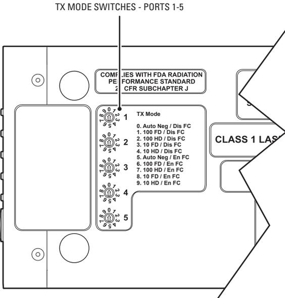
**Figure 4.** TX Mode Switches for 10BASE-T/100BASE-TX Ports 1-5
