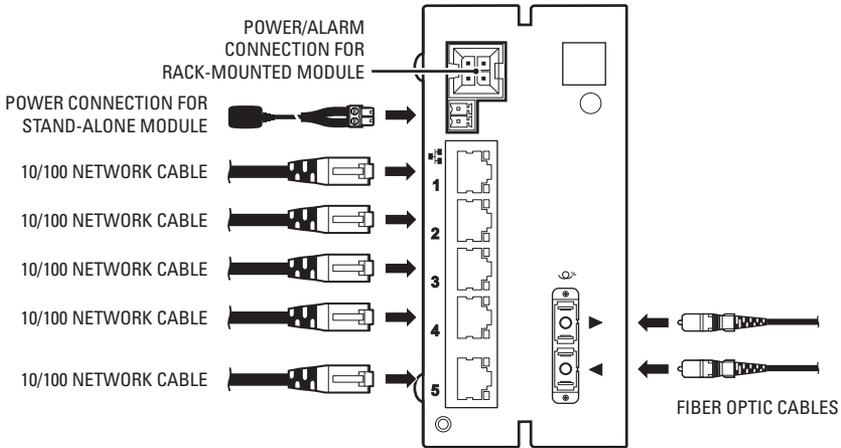
**Figure 6. FX82051 Module Connections**
