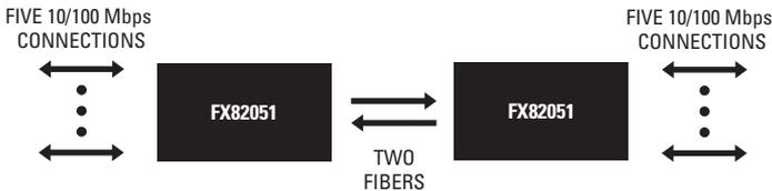
**Figure 1.** FX82051 Point-to-Point Application
