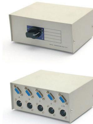
StarTech.com's Manual 4-to-1 VGA/SVGA Monitor Switchbox lets up to 4 computers share 1 monitor or 1 keyboard. Requiring no power supply, this switchbox is ideal to sit on a user's desktop and allow them to manually switch between active computers.
