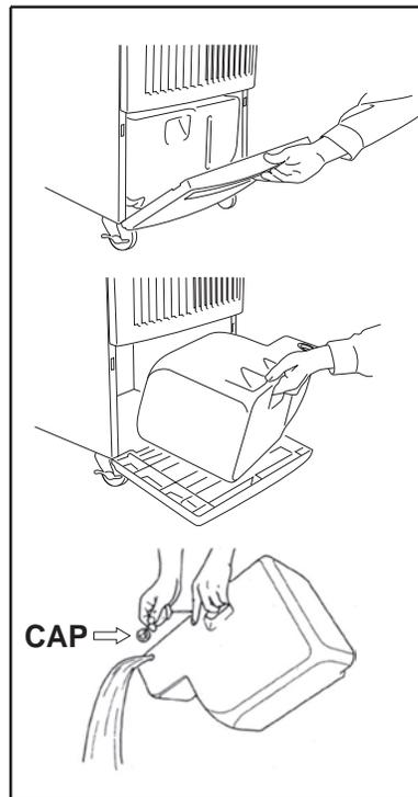
4) Replace the cap and return the drain tank to the unit.
