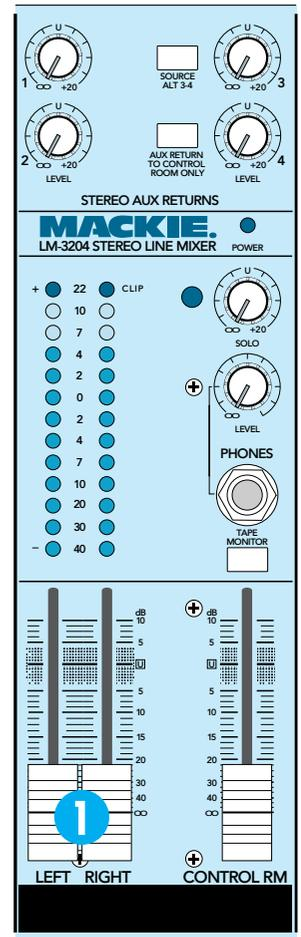
0dBu (.775 volts rms) at the rear output jacks. The LM-3204's main outputs are 0dBu=0dB Meter whether you are using balanced or unbalanced cables.
