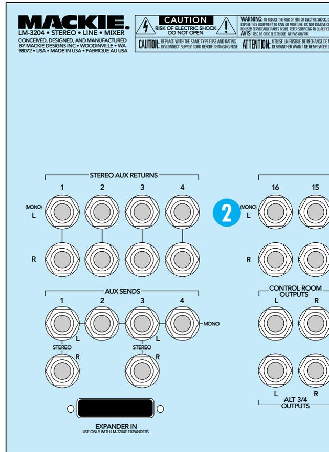
2. As a "direct output," which also interrupts the signal to the output section. Use a 1/4" TS (mono) plug, and push it in all the way to the second click.
