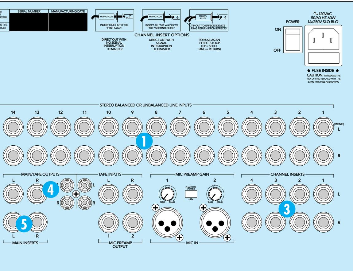
**3.** As a send-return insert for processing. Use a 1/4" TRS (stereo) plug "Y"-ed to two mono (TS) 1/4" plugs. The tip should be wired to send to the effect's input, and the ring should be wired as the return from the effect back into the LM-3204. The sleeve is the common ground connection.
