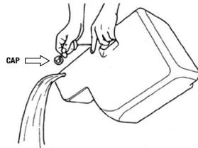
④ Replace the cap and return the drain tank to the unit.
