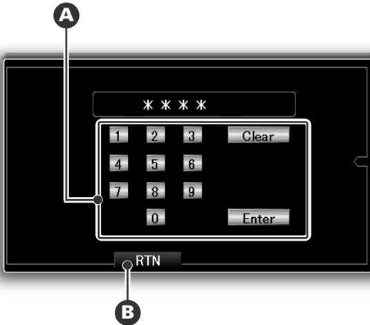
**When the battery is removed from the unit's power switch, you cannot turn on the unit again unless the preset security code is input. This function helps prevent theft.**
