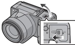
**2** **Battery:** Being careful about the battery orientation, insert all the way until you hear a locking sound and then check that it is locked by lever (A). Pull the lever (A) in the direction of the arrow to remove the battery.
