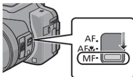
**3** Slide the side lever to display focus range on the screen.
