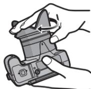
**3** You will feel some stiffness just before the mark, but continue to rotate the lens hood to **A** where the marks align. (The lens hood will stop with a “click”.)
