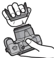
**2** Rotate the lens hood in the direction of the arrow.
