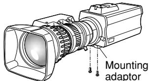
Use a screwdriver or similar to tighten the screws to secure the mounting adaptor. Make sure that the mounting adaptor is attached the right way round.
