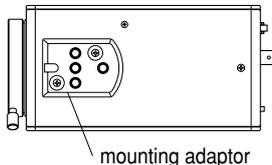
2. Fix the camera mounting base, pan/tilt unit, and tripod securely in the screw hole (1/4-20UNC) of the camera or the mounting adaptor.
