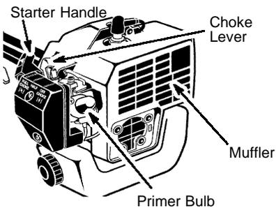
5. Pull starter rope handle sharply until engine sounds as if it is trying to start, but do not pull rope more than 6 times.
