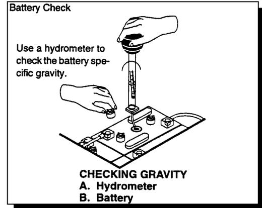
To find the correct specific gravity reading when the temperature of the battery electrolyte is other than 80° F (27° C).
