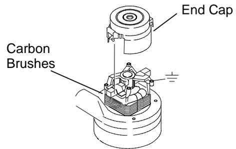
If armature commutator is grooved, extremely pitted or not concentric, the motor will need to be replaced or sent to a qualified service center.
