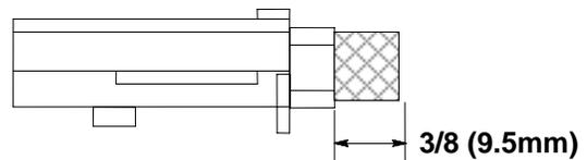
Periodically check the length of the carbon brushes. Replace both carbon brushes when either is less than  $\frac{3}{8}$ " (9.5mm) long.
