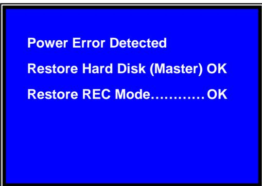
If a power error occurs during recording process, the system will automatically resume recording after power is reconnected.
