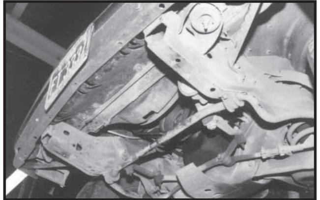
6. Raise base plate and make sure pulling ears clear Air Dam/Valance slots. Use base plate for template and mark front holes. Remove base plate and frame nut strip.
