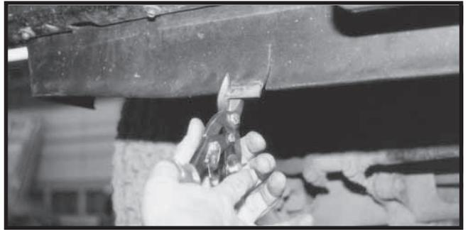
5. Lower or completely remove base plate. Cut out air dam/valance slots as earlier marked. Trial fit the base plate.
