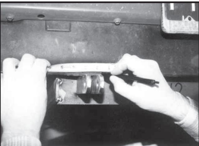
4. Mark the 1-5/8" x 2-1/2" slots by using the pulling ears of the base plate to guide you in the location.
