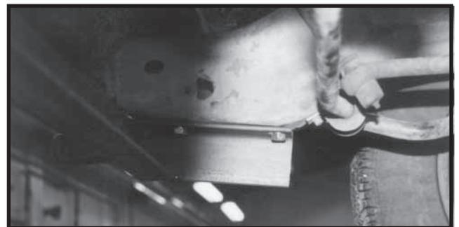
8. Install base plate and nut strip using four 1/2" x 1-1/2" bolts and 1/2" lockwashers. **NOTE: *LOCTITE* Blue must be used on all fasteners.**
