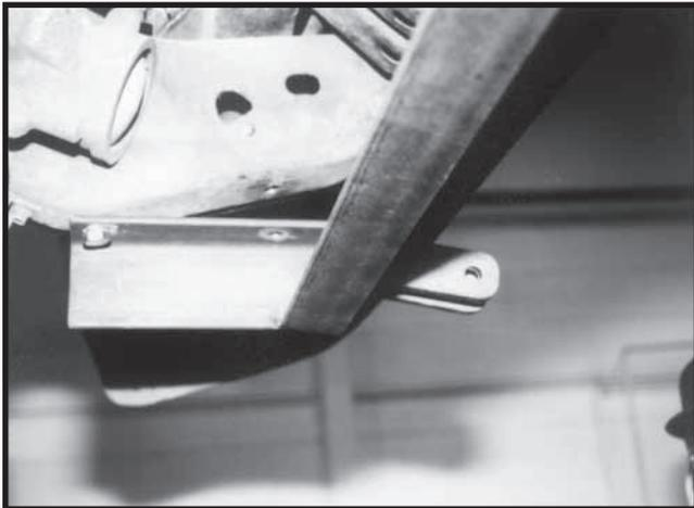
3. Install base plate with rear bolts snug so front ears touch Air dam/Valance. **NOTE: Some bolts may need to be put back in so it is stable for marking and cutting of slots.**
