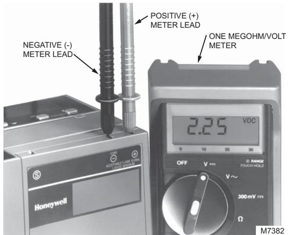
**Fig. 5. Measuring 7800 SERIES Control flame signal voltage.**
