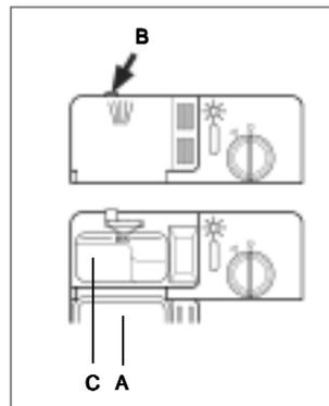
**Note: To facilitate closing the cover, remove any excess detergent on the edges of the dispenser.**
