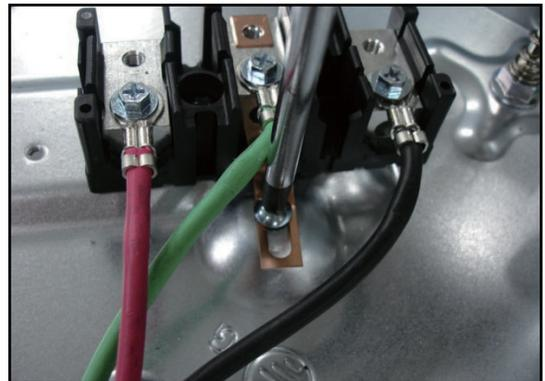
3. Loose the ring of conduit bracket with a hand to remove the power cord assembly.
