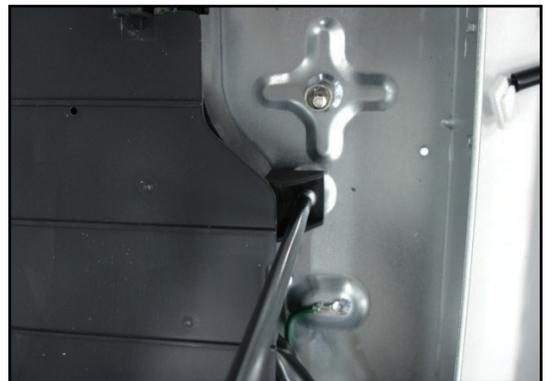
4. Lift the front side of burner assembly and take out IH module assembly.
