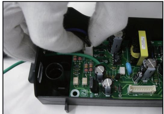
3. Cut out the hook as below. (This is not a problem when reassembling. It can be fixed without that.)
