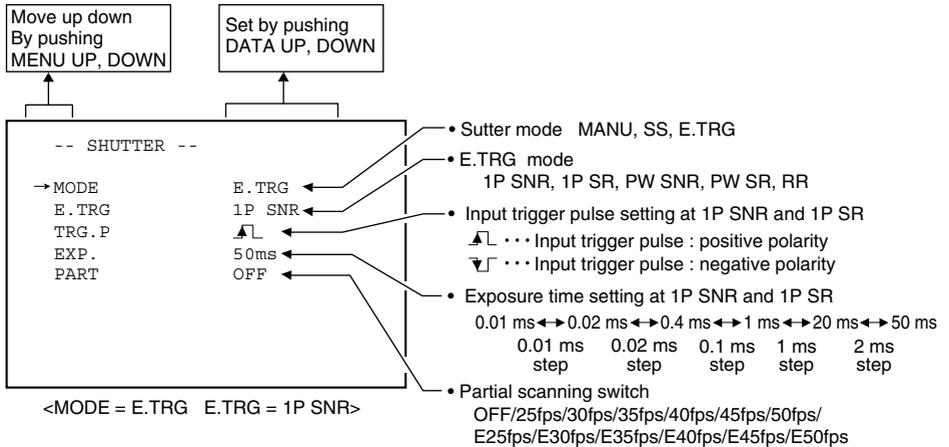
**(a) Changing the polarity of inputting trigger pulse setting**
