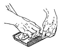
Turn unit around. Pull back clip and insert other end of screen. See figure 3.
