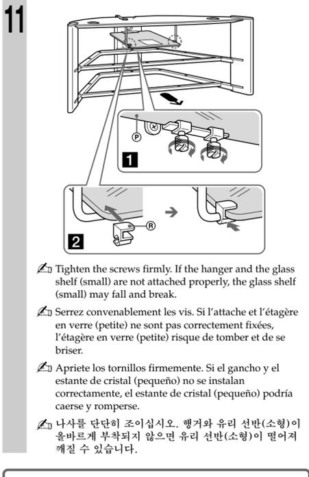
Tighten all of the assembly screws correctly.
