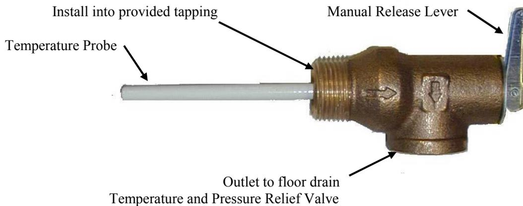
3. Install a relief valve overflow pipe to a nearby floor drain. CAUTION: No valve of any type should be installed between the relief valve and tank or in the drain line.
