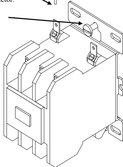
5. Replace with new contactor using reverse procedure.
