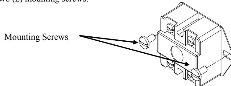
5. Replace control and install new high limit switch by performing above steps in reverse order. See wiring diagram included with drawing for assistance.
