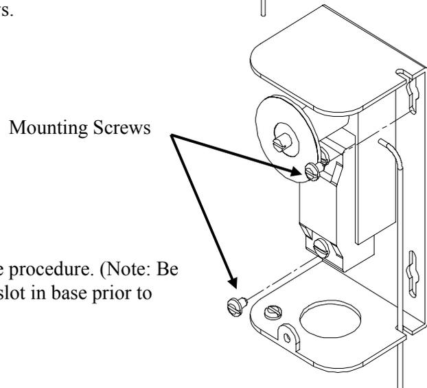
7. Replace thermostat using reverse procedure. (Note: Be sure to place capillary tube into slot in base prior to installing cover.)
