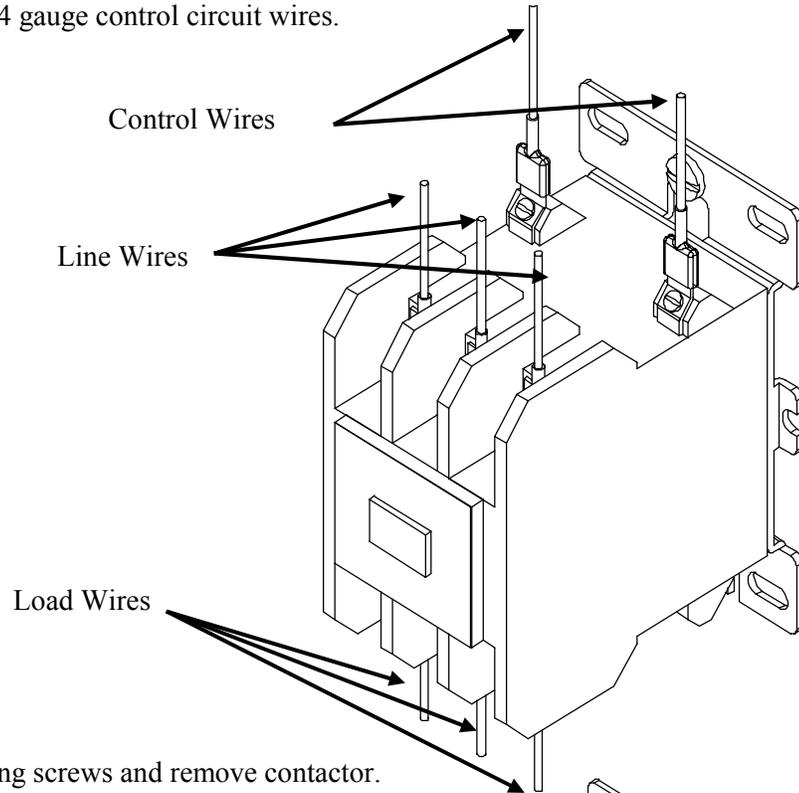
4. Loosen two (2) holding screws and remove contactor.
