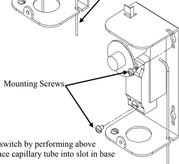
7. Remove control and install new high limit switch by performing above steps in reverse order. (Note: Be sure to place capillary tube into slot in base prior to installing cover.)
