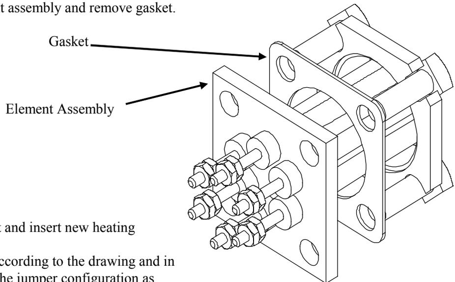
9. Install new gasket and insert new heating element.
