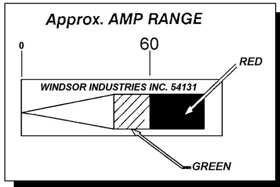
1. Connect a DC ampere meter to the positive battery lead. Running the machine with a pad, lower the pad to the floor until it is operating at 55-60 amps.
