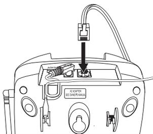
5. Plug the other end of the cord into the telephone jack on the wall.
