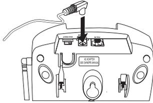
2. Place the AC Adapter cord inside the molded channel.
