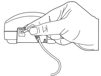
2. Place the AC Adapter cord around the strain relief.
