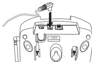
3. Place the AC Adapter cord around the strain relief.
