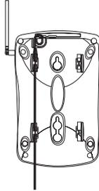
3. Plug one end of the short telephone cord into the TEL LINE jack on the Base Unit.
