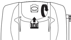
3. Put the retainer back into its slot on the Base Unit.
