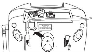
4. Plug one end of the long telephone cord into the TEL LINE jack on the Base Unit.
