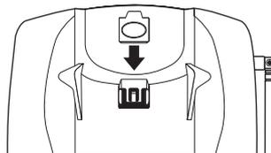
4. Push down on the Handset retainer until it snaps into place.
