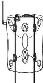
6. Place the Base Unit on the screws and push down until it's firmly seated.
