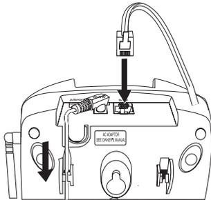
4. Place the telephone cord inside the molded channel on the bottom of the Base Unit. Then plug the other end of the telephone cord into the modular jack on the wall.
