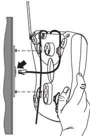
5. Place the Base Unit on the posts of the wall plate and push down until it's firmly seated.
