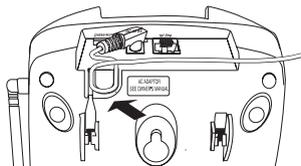
**Important:** Place the power cord so that it does not create a trip hazard, or where it could become chafed and create a fire or other electrical hazards.
