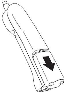
3. Align the plastic connector of the Nickel-Cadmium battery pack with its socket and plug it in.
