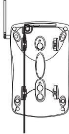
4. Plug one end of the long telephone cord into the TEL LINE jack on the Base Unit.
