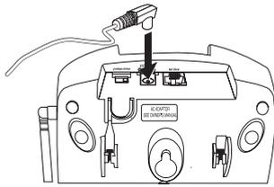
3. Place the AC Adapter cord inside the molded channel.
