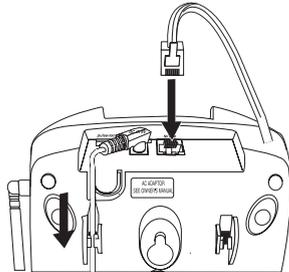
5. Place the cord inside the molded channel on the bottom of the Base Unit.
