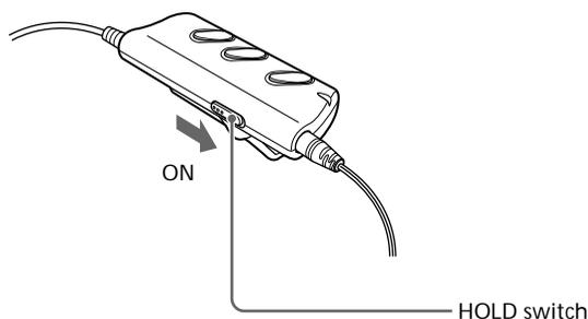
Sliding the HOLD switch of the Audio Adapter to ON, you cannot use the buttons of the Audio Adapter, but you can use the buttons of the CLIÉ handheld itself.
