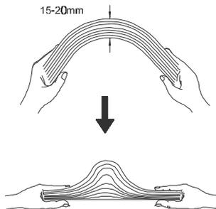
Take a 2 to 4 mm thickness of sheets. Lightly hold both ends with both hands. Bend the sheets as shown. Hold the sheets tightly with both hands then straighten the sheets. This operation separates the sheets for easy feeding into the ADF. Repeat this operation two or three times. Turn the stack of sheets over and repeat the entire operation.
