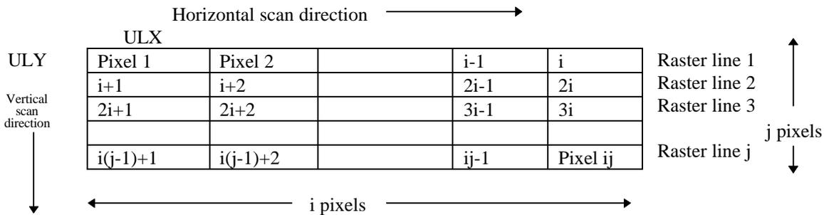
The following format is the data format that this scanner uses when transferring the image data of a window comprising  $i \times j$  pixels.
