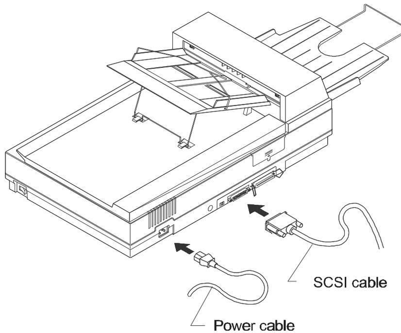
**Figure 3-3 Signal cable connection**
