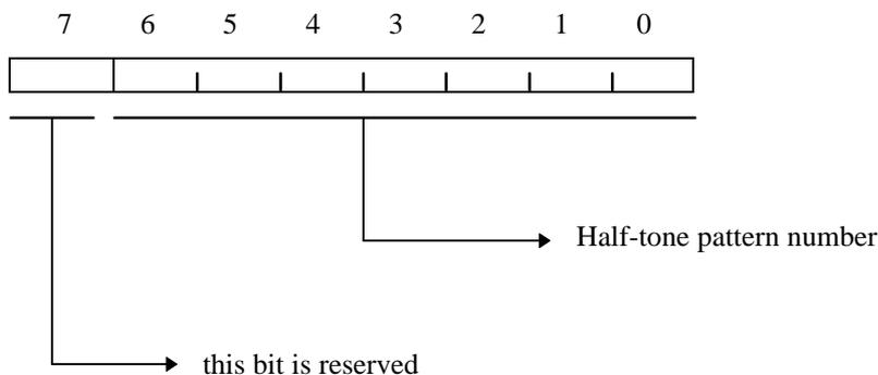
This scanner has four types (X'00' to X'03') of built-in pattern. If a value greater than the four range is specified, this scanner returns the following error:
