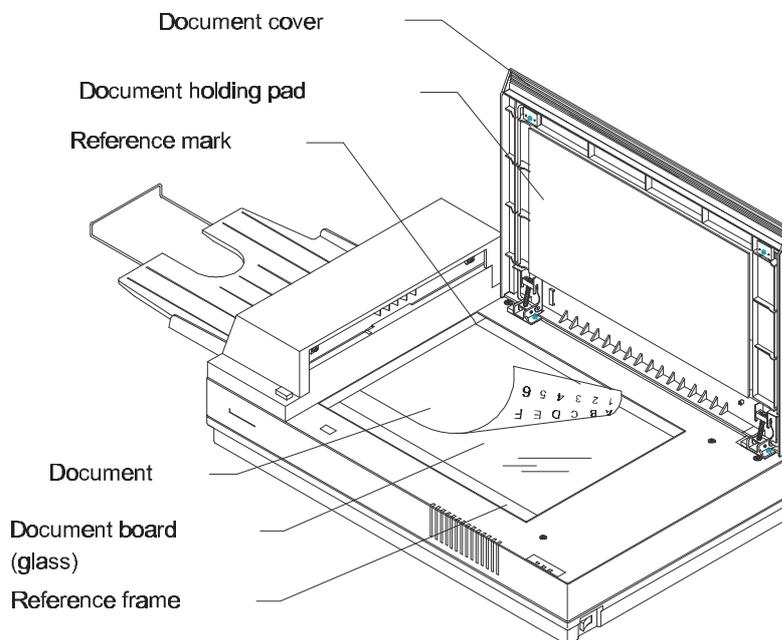
**Figure 3-6 Flatbed reading**
