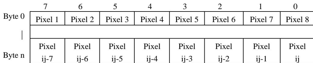
If the data amount per raster line is not a multiple of 8 bits, the window is raised to a multiple of 8 bits.
