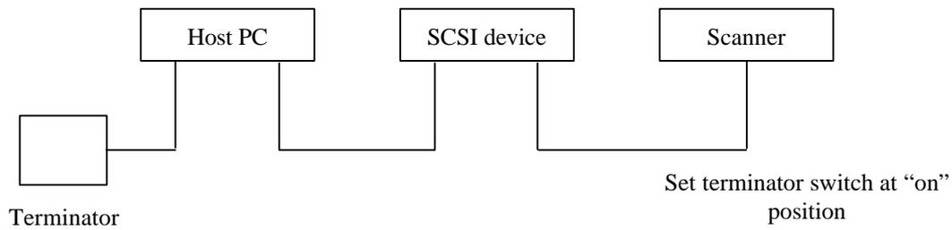
If there is already another device linked to the host via SCSI cable, remove the terminator from that device. If the terminator can not be removed, it is recommended that the connection of Configuration I be used.
