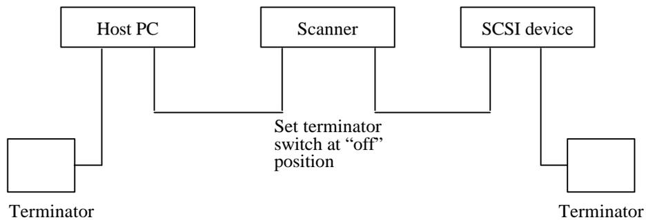
1. Set scanner's SCSI terminator switch off.
