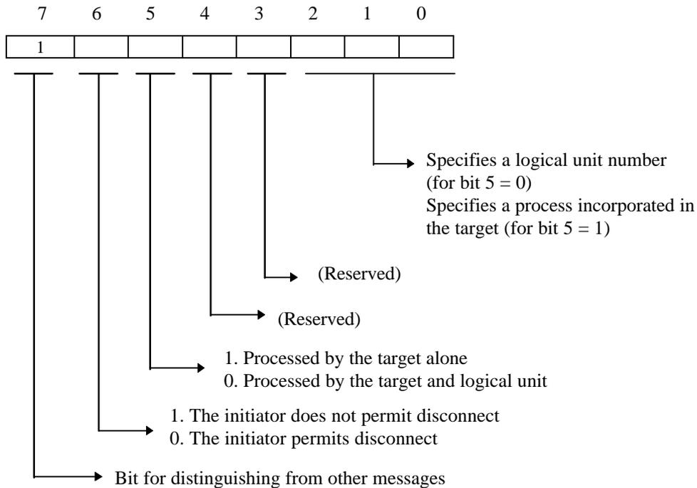
This scanner does not support the target-incorporated process function. Therefore, if a 1 is set in bit 5, the IDENTIFY message is rejected with the MESSAGE REJECT message.
