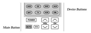
**Example:** To set-up the remote to operate a TV, press the TV *Device Button* and the *Mute* button, simultaneously.
