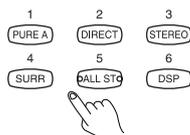
**PURE AUDIO (PURE A) (TX-SR700/700E only):** Changes the listening mode for the signal type that is currently being input from the selected input source to the Pure Audio listening mode. If pressed, the corresponding setting in the “Input Setup” menu for the selected input source is also changed (see page 54).
