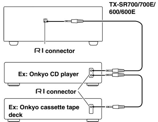
To connect components using the **RI** terminal, simply connect a remote control cable from this **RI** terminal to the **RI** terminal of the other component. An **RI** remote control cable with a 1/8-inch (3.5-mm) miniature two-conductor plug comes with every cassette tape deck, compact disc player, MD recorder, and DVD player that has an **RI** terminal.
