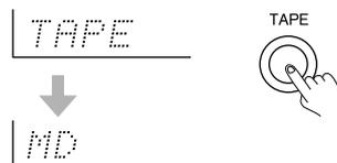
To return the display to its original setting, perform the same procedure. This setting is necessary to allow **RI** system functions for a connected Onkyo cassette tape or MD recorder.
