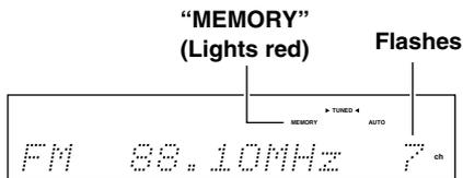
3. Using the PRESET buttons, select a preset number (from 1 to 40) to assign the station.
