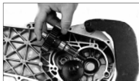
If this seal is damaged, oil will flow to the outside through the outlet slot located in the return spring housing of the brake key; Photo opposite.
