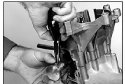
The opening of the snap ring will be positioned at the top or at the bottom, but under no circumstances to the side.
