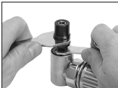
Figure 2. Loosening the collet.
