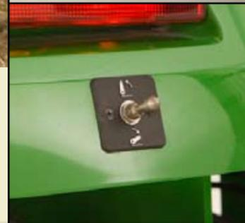
External raise/lower switch, located on the rear fender, lets you adjust the 3-point hitch while outside of the cab for easier hookups.
