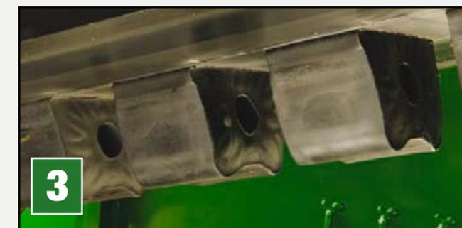
(1) New mid rollers are 1.25 inches wider than previous models to help reduce slippage and increase belt tension. (2) Twin nitrogen accumulators and a larger tensioning cylinder increase track belt tension by 20 percent. (3) New guide lugs are 36 percent larger than previous models. These improvements help reduce track belt wear and improve tractor performance on steep hillside applications.
