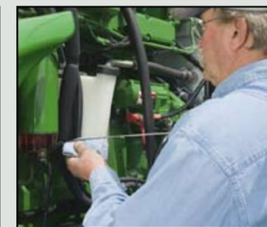
**Access to common service check points** is unobstructed making daily oil and coolant level checks quick and easy.
