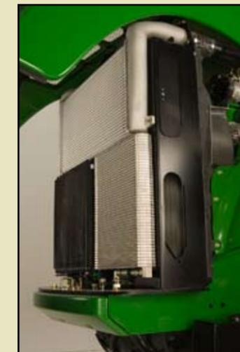
**New radiator** is 29 percent larger than previous models for increased cooling capacity.
