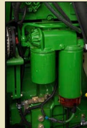
**New self-priming fuel system** eliminates messy hand priming and filter pre-filling for fast, easy filter changes.
