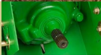
A 20-spline, 1¾-in. diameter, 1,000-rpm PTO is optional for the 9330, 9430, and 9430T.
