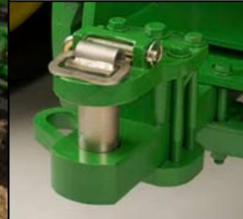
A new Category 5 drawbar is standard on the 9530, 9530T, 9630, and 9630T. A 12,000-lb. vertical-load carrying capacity, and massive 2.75-inch hitch pin, give you the added capacity to pull heavy or extra-wide implements.
