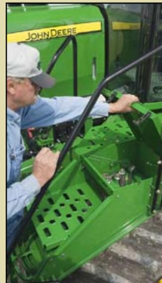
A new toolbox is built into the platform (left) for easy access and for storage of tools, chains, or other equipment. **New track-alignment mechanism** (right) makes adjustments easier and improves belt tracking.
