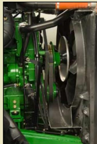
**Field-proven Vari-Cool™ system with variable-speed fan drive** automatically adjusts its speed to keep the engine and hydraulic system cool. It also improves fuel economy and boosts pulling power.
