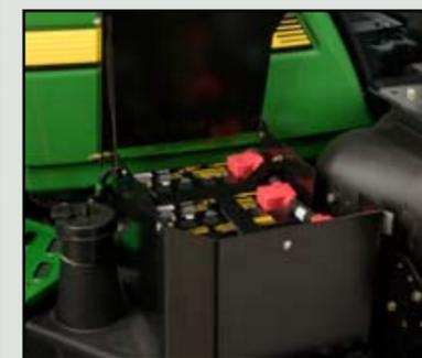
**Flip-up battery cover** features an air cylinder to hold it up during periodic inspections or annual service.
