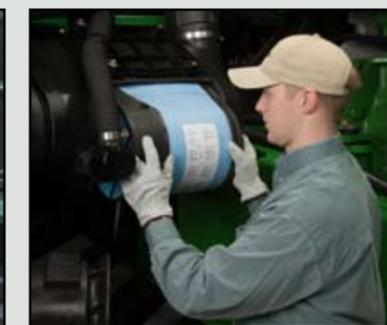
**Annual air filter replacements** are a breeze for all 9030 Series tractors. Filters can be conveniently reached while standing on the ground.
