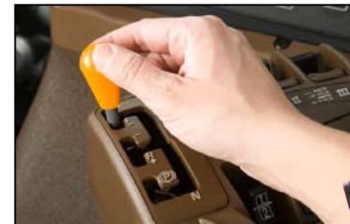
The convenient shift lever on the CommandARM console lets you smoothly move through 18 forward or six reverse gears with just your thumb. Easily shift into park, neutral, forward, or reverse, as well as change gears up or down. Transport up to 24 mph (4WD).
