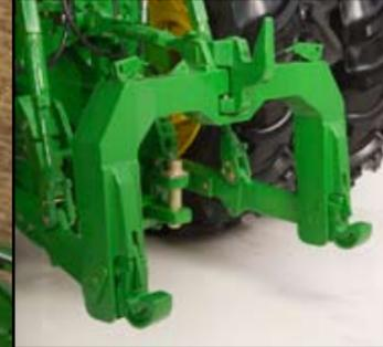
Hitch-lift capacity has been increased to 15,300 lb. A 3-point rear hitch with Quick-Coupler is available on all models as a factory or field-installed option.
