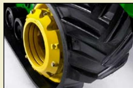
A new 60-degree drive wheel pattern (right) grips the track belt more efficiently, reducing slippage for better performance.
