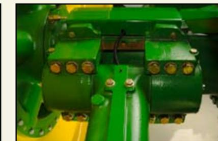
(5) Heavy-duty damping cylinder (left) provides additional cushion as the walking beam travels vertically.
