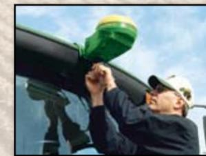
**StarFire™ iTC™ position receiver** with Integrated Terrain Compensation corrects all position calculations to adjust for uneven ground and slopes.
