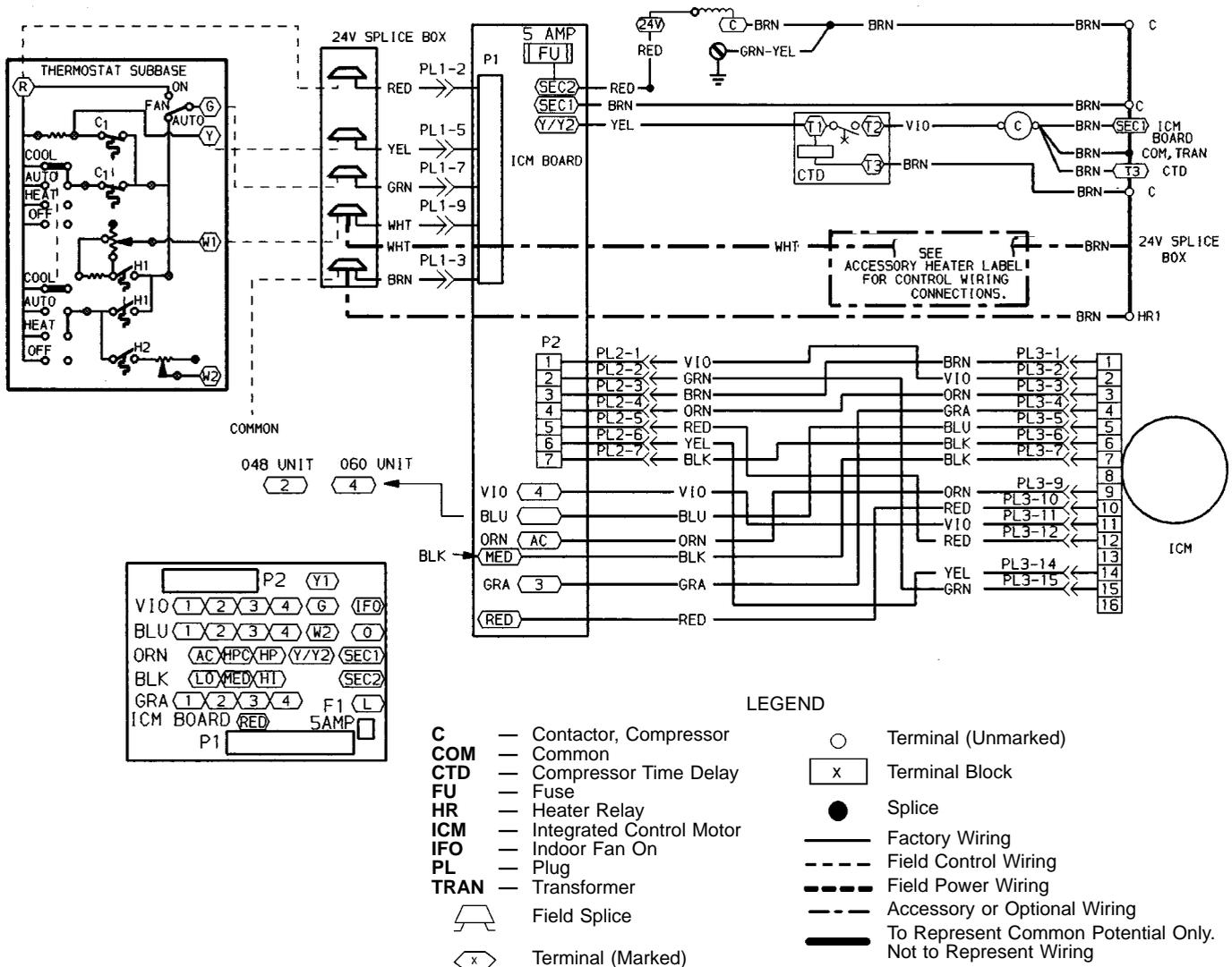
**Fig. 33 — Units 50SX048,060 — 208/230-1-60, Integrated Control Motor Wiring Schematic**
