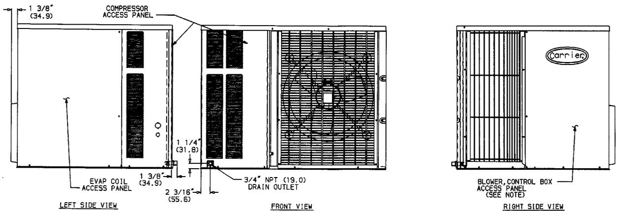
Fig. 8 — Dimensions; Units 50SX042-060 Without Base Rail
