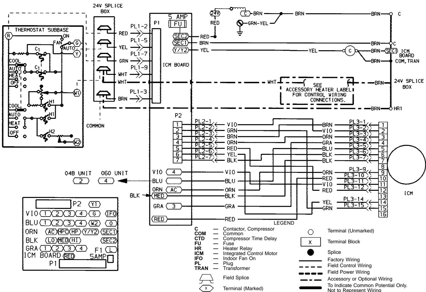
Fig. 34 — Unit 50SX048,060 — 208/230-3-60 Integrated Control Motor Wiring Schematic
