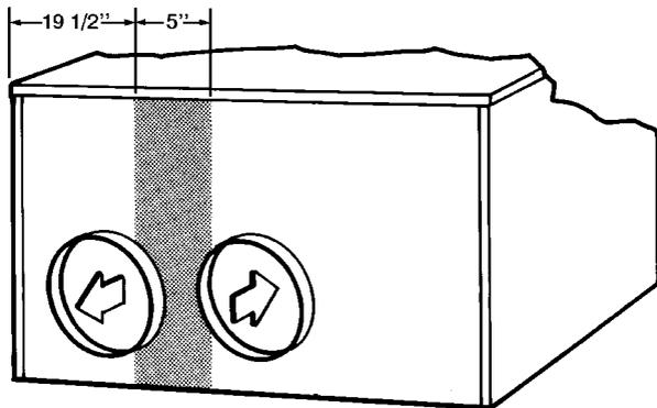
**Fig. 13 — Area Not To Be Drilled**
