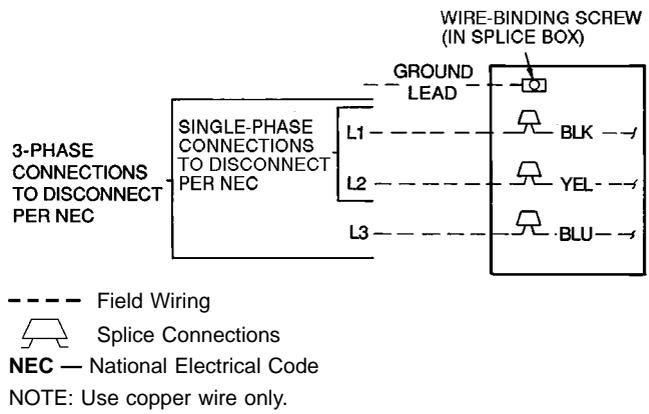
**Fig. 30 — Line Power Connections**
