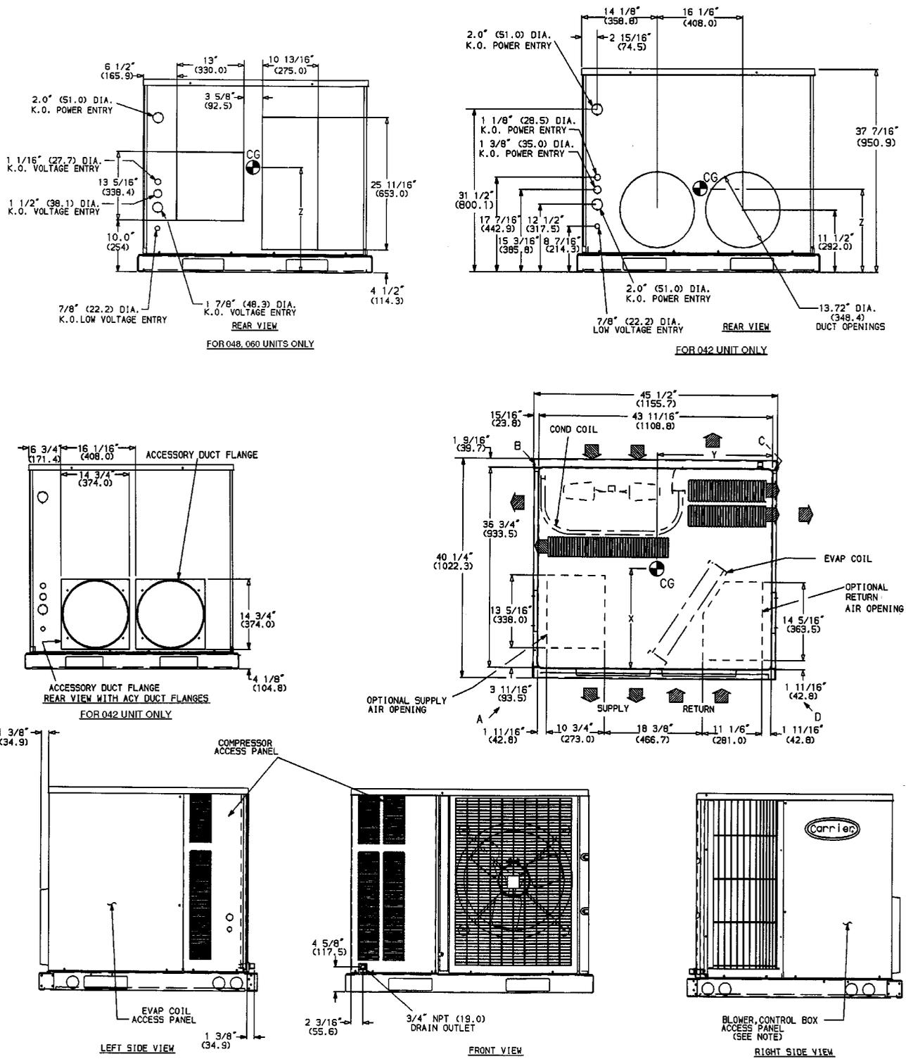
**Fig. 9 — Dimensions; Units 50SX042-060 With Optional Base Rail**
