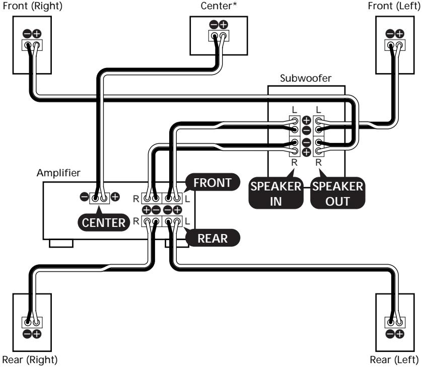
\* (SA-VE505 only) Connect the center speaker to the amplifier and mount it onto the supplied speaker stand for placement on the top of the TV set (see page 7).
