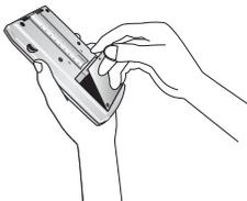
**3 Use a pen or other sharp instrument to press the reset button located in the hole to the right (above the battery).**
