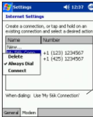
*After you select the modem card connection for dialing, it should be identified here.*
