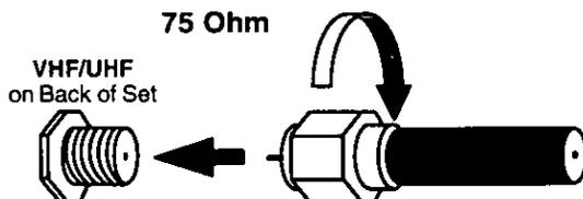
**NOTE:** Certain cable systems offset some channels to reduce interference or have Premium (scrambled) channels. A cable converter box is required for proper reception. Check with your local Cable company for compatibility requirements.
