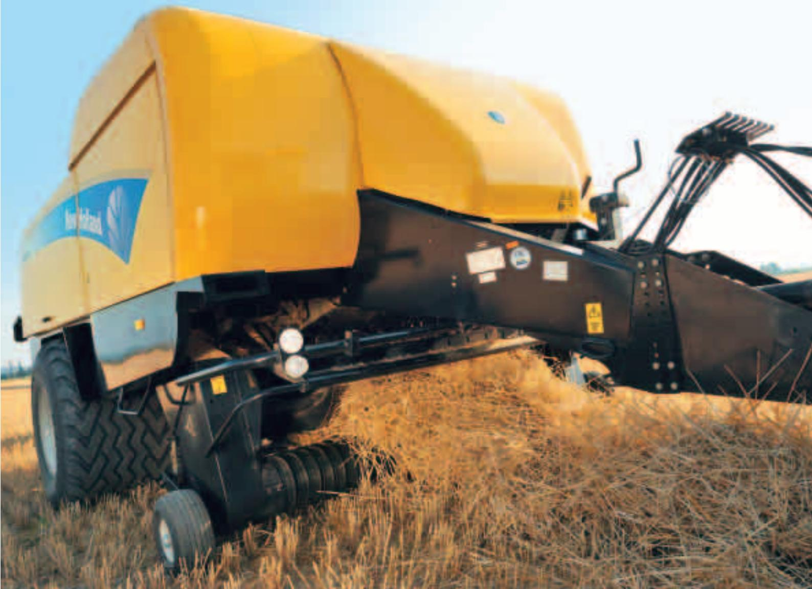
Even the shortest piece of straw or the smallest dry leaf of valuable hay is taken up by the Super Sweep™ pick-up. Proven characteristics like curved tines and close tine spacing combined with an efficient wind-guard and pneumatic gauge wheels help to sweep fields clean at a high speed.
