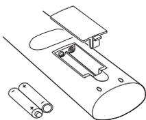
Remove the back cover to insert the batteries, make sure they are inserted the right way round.
