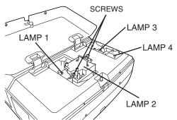
Make sure which number of lamp needs to be replaced on Lamp Status Display. Figure shows case of replacing LAMP 2.
