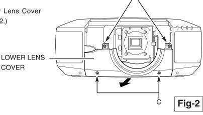
Remove 2 Screws D and Cover Plate on the back of Upper Lens Cover. (See Fig. 3.)
