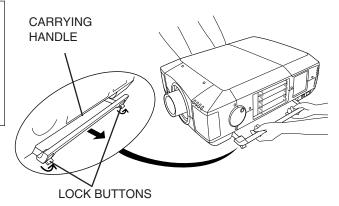
Pull up lock buttons to release lock.
