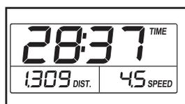
**The lower right display**—The lower right display can show the speed of the walking belt and the approximate number of calories that you have burned.
