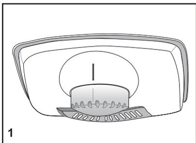
Operating temperatures are controlled by the thermostat (see diagram) located on the ceiling of fridge compartment. Settings may be made from 1 to 5, 5 being the coldest position.
