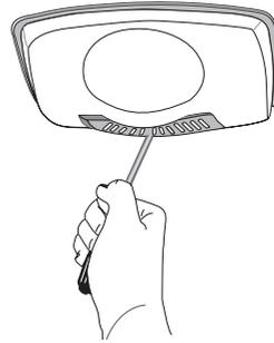
3. First check that the bulb hasn't worked loose by ensuring it is screwed securely in the holder. Replace the plug and switch on. If the bulb works, replace the light cover by inserting the rear lug and pushing up to locate the front two lugs.
