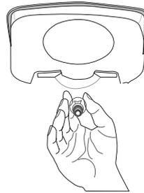
4. If the light still fails to work, switch off at the socket outlet and pull out the mains plug. Replace the bulb with a new 15 watt (max) screw cap (SES) bulb.
