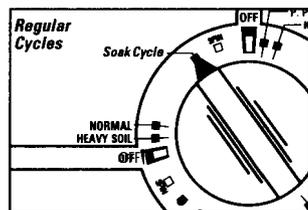
Start the washer. After washer fills and begins to agitate, push in the Cycle Selector knob and turn to SOAK CYCLE. Pull out the Cycle Selector knob to complete the cycle.
