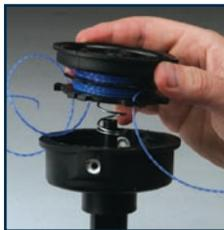
9. When operating for the first time after changing the spool of line ensure to test the assembly by running the line trimmer in a safe location. The line may not be fully extended so you may need to “bump” the head at full speed to feed the line to the correct length.
