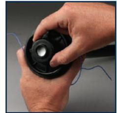
anti-clockwise, as indicated by the “OFF” arrow, to unscrew it from the trimming head (6).
