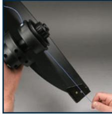
**WARNING.** For your own safety when adjusting the length of the line, avoid coming into contact with the line cutting blade (8) which is fixed to the guard. It is extremely sharp. Keep your hands well away from this area.
