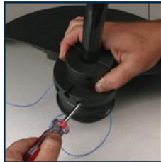
5. Fit the secondary handle (4) to the upper shaft (23) by fitting the handle over the shaft and placing the locking clamp nut (included) through the holes in the guard and tightening in the most comfortable position to the secondary handle locking knob (16).
