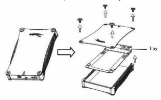
2 Place the hard drive into the tray, connecting the data connector to the corresponding connector on the printed circuit board, then secure the drive to the tray with four screws (provided).
