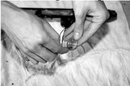
8. Now hold the LED assembly centered over the hole where the original bulb was and align the mounting plate from the bottom with the slot in the housing. Position the LED assembly so the screw holes line up.
