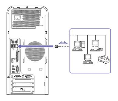
Connect only 10BASE-T/100BASE-TX cables to the Ethernet port. Using other cables or a telephone cable may cause a malfunction, excessive heat or even fire in the port. If using this computer in Germany, please make sure you do not use an ISDN cable. It is physically very similar, but its higher voltage of 12V may destroy the motherboard inside the computer.
