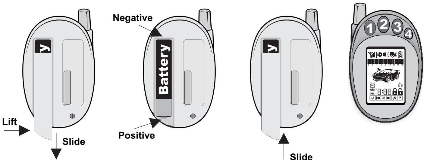
**Note- Avoid reinstalling the battery in the wrong direction**
