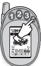
1. Press and release Button #4 while the vehicle is running by the ignition key.
