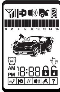
**STATUS CHECK MODE** This feature is used to check the status of the alarm system or the remote starter.
