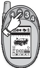
1. Press and hold Button #2 (Optional to button #4\*) for three seconds.
