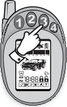
1. Press and release Button #3 on the remote transmitter.
