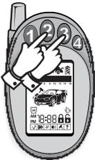
1. Press and hold buttons #2 & #3 together for two seconds.
