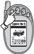
1. Press and release button #1 on the remote transmitter. The park lights will flash, the horn (optional) will honk twice and the doors will lock.
