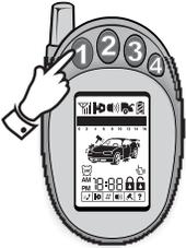
1. Press and release button #1 on the remote transmitter. The park lights will flash, the horn (optional) will honk one time and the doors will lock.
